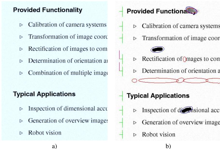
Figure 98: Cut-out of the reference and the checked test image with the differences marked in the test image: a) Reference image; b) checked test image.
