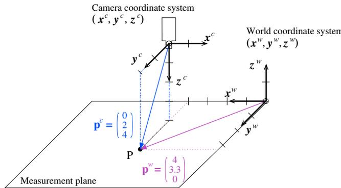
Figure 3: Coordinates of a point in two different coordinate systems.
