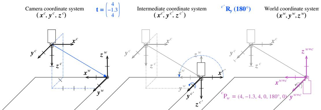
Figure 10: Determining the pose of the world coordinate system in camera coordinates.
