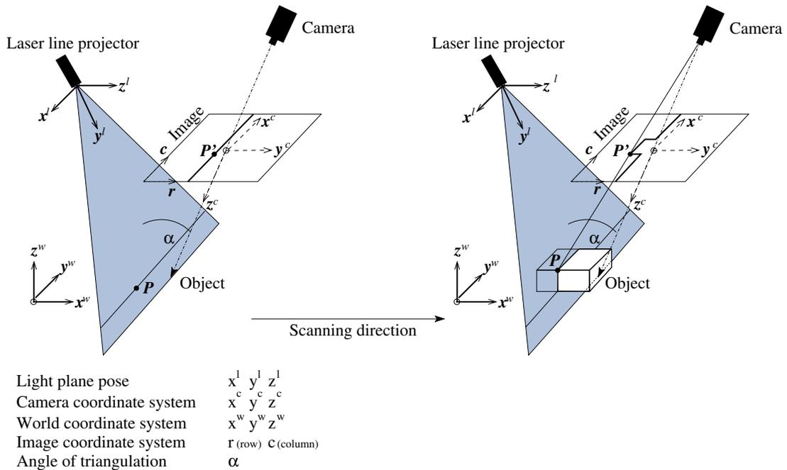
Figure 99: Basic principle of sheet of light (light plane marked in gray).
