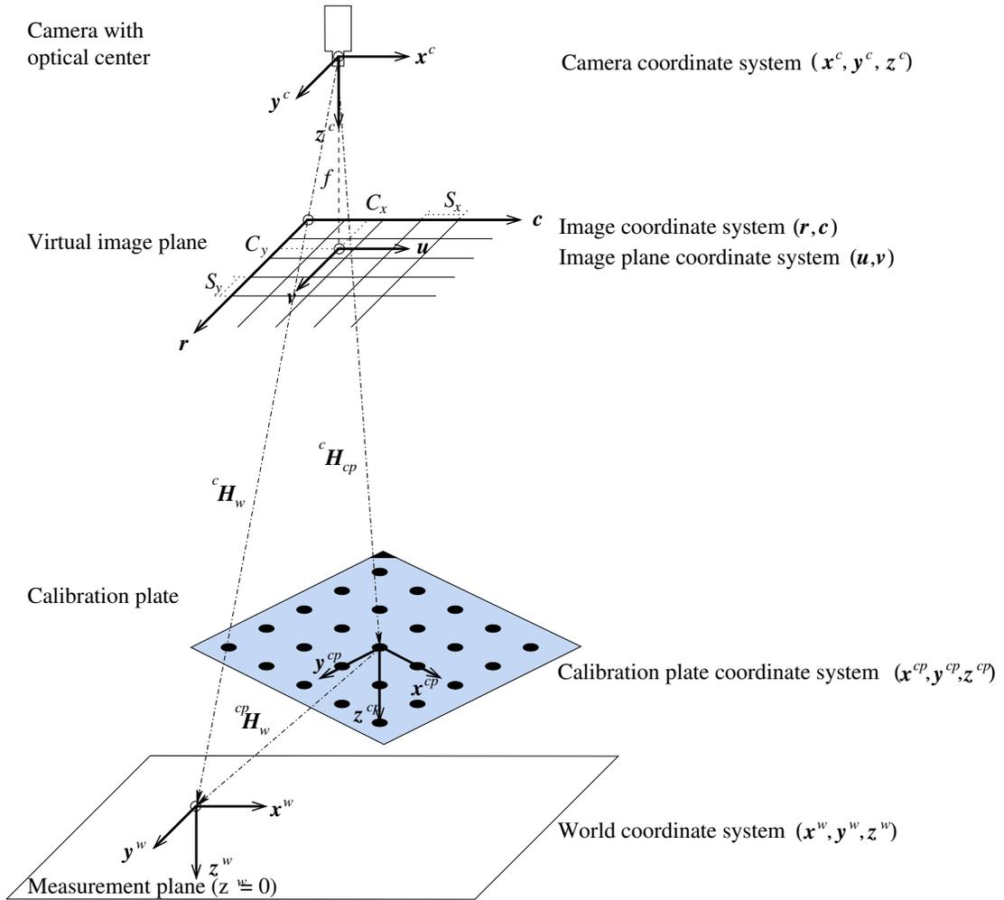
Figure 25: Relation between calibration plate and measurement plane.
