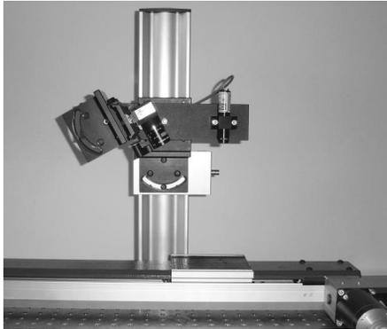
Figure 102: Exemplary setup for a sheet-of-light measurement consisting of a camera, a laser line projector, and a positioning system.
