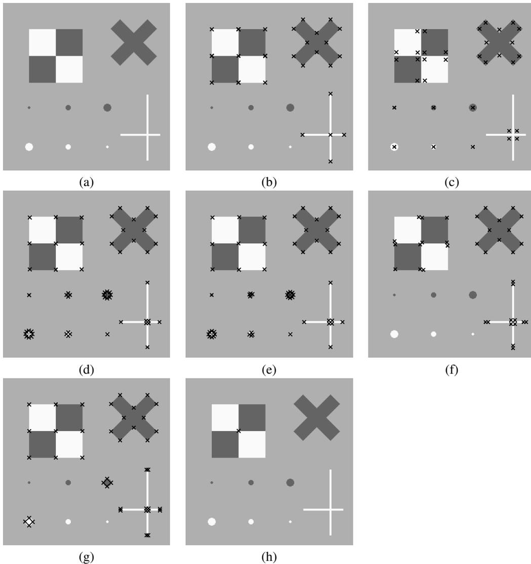
Figure 55: Comparison of typical results of interest operators. a) Test image; b) Förstner, junctions; c) Förstner, area; d) Harris; e) Harris, binomial; f) Lepetit; g) Sojka; h) Saddle points.
