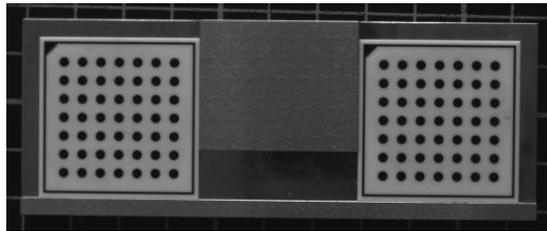
Figure 34: Calibration object for two-camera setup.
