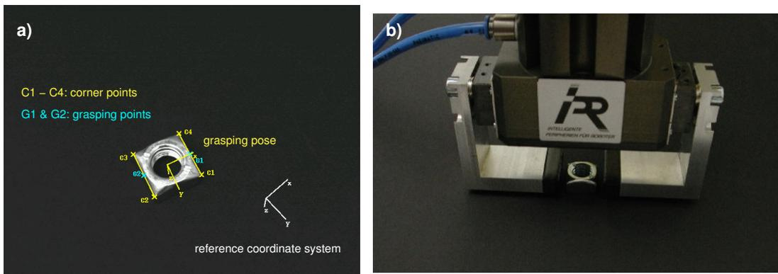
Figure 84: (a) Determining the 3D pose for grasping a nut; (b) robot at grasping pose.
