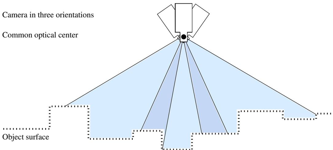
Figure 47: Image acquisition for non-flat objects.
