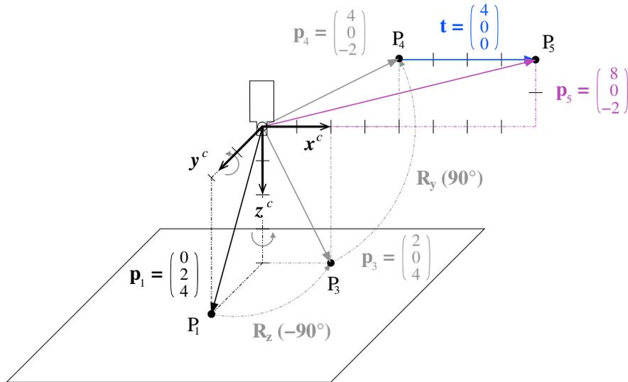
Figure 9: Combining the translation from [figure 4](#) on page 9 and the rotation of [figure 6](#) on page 11 to form a rigid transformation.
