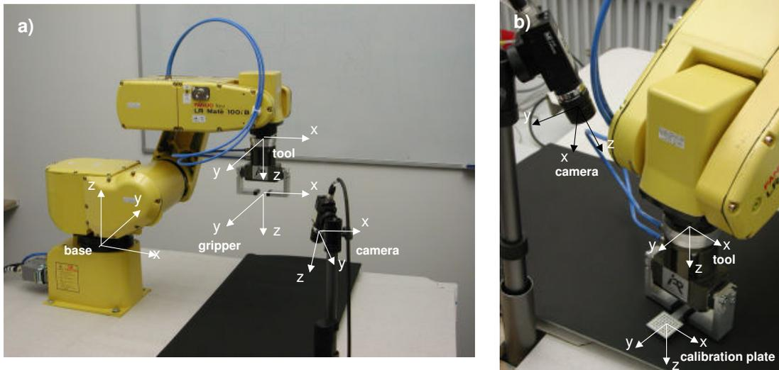
Figure 83: Example hand-eye system with a stationary camera: coordinate systems (a) of robot and camera, (b) with calibration plate.
