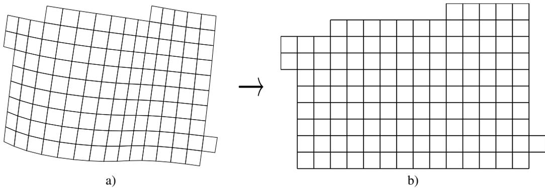
Figure 89: Mapping of the distorted rectification grid (a) into the undistorted rectification grid (b).
