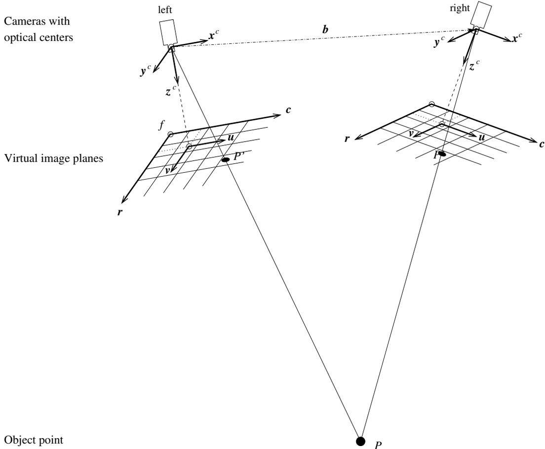
Figure 66: Stereo camera system.
