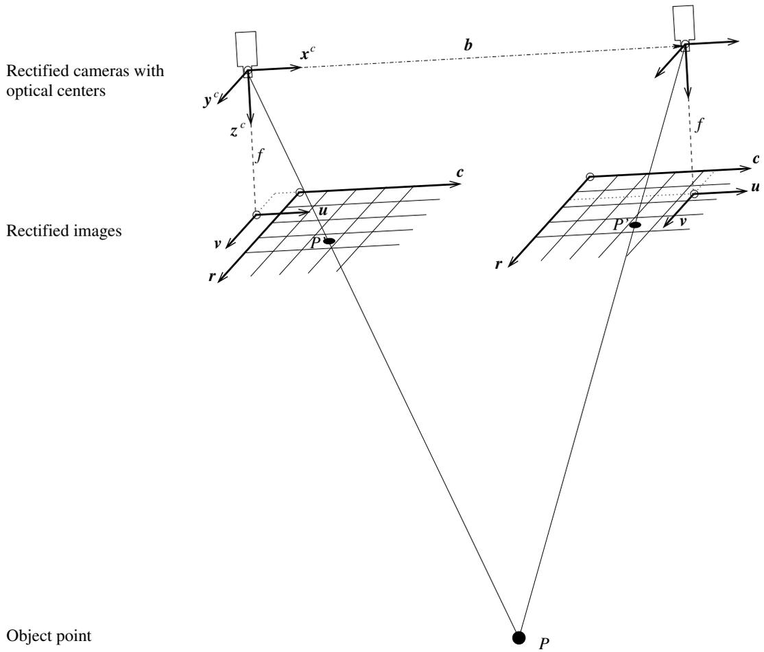
Figure 73: Rectified stereo camera system.
