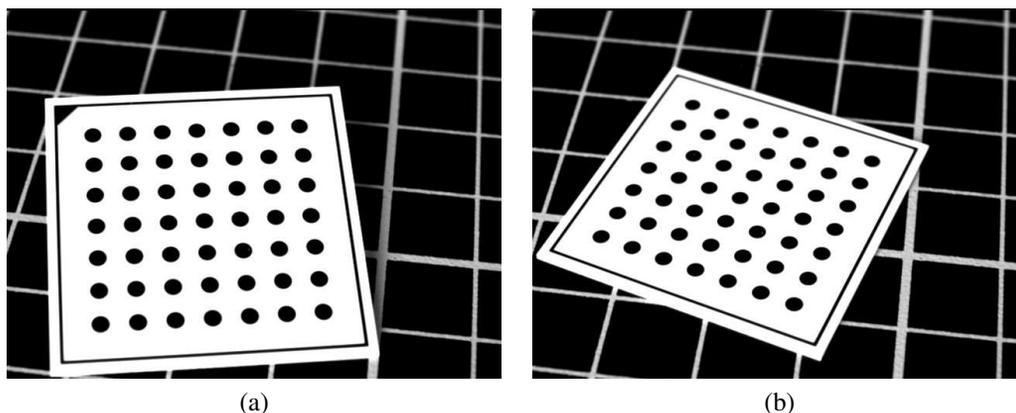
Figure 113: (a) The HALCON calibration plate with the asymmetric pattern in the upper left corner; (b) an old calibration plate that does not have the asymmetric pattern.
