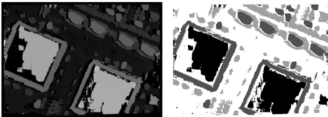
Figure 79: Left: Height above the reference plane; Right: Segmentation of high objects (white: 0-0.4 mm, light gray: 0.4-1.5 mm, dark gray: 1.5-2.5 mm, black: 2.5-5 mm).
