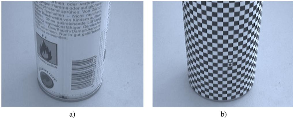
Figure 92: Cylindrical object: a) Without and b) with rectification grid.
