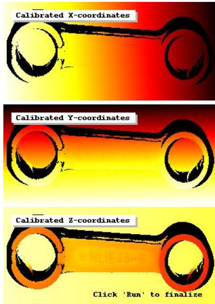
Figure 109: Result of calibrated sheet-of-light measurement: images representing the (from top to bottom) x, y, and z coordinates of the object.
