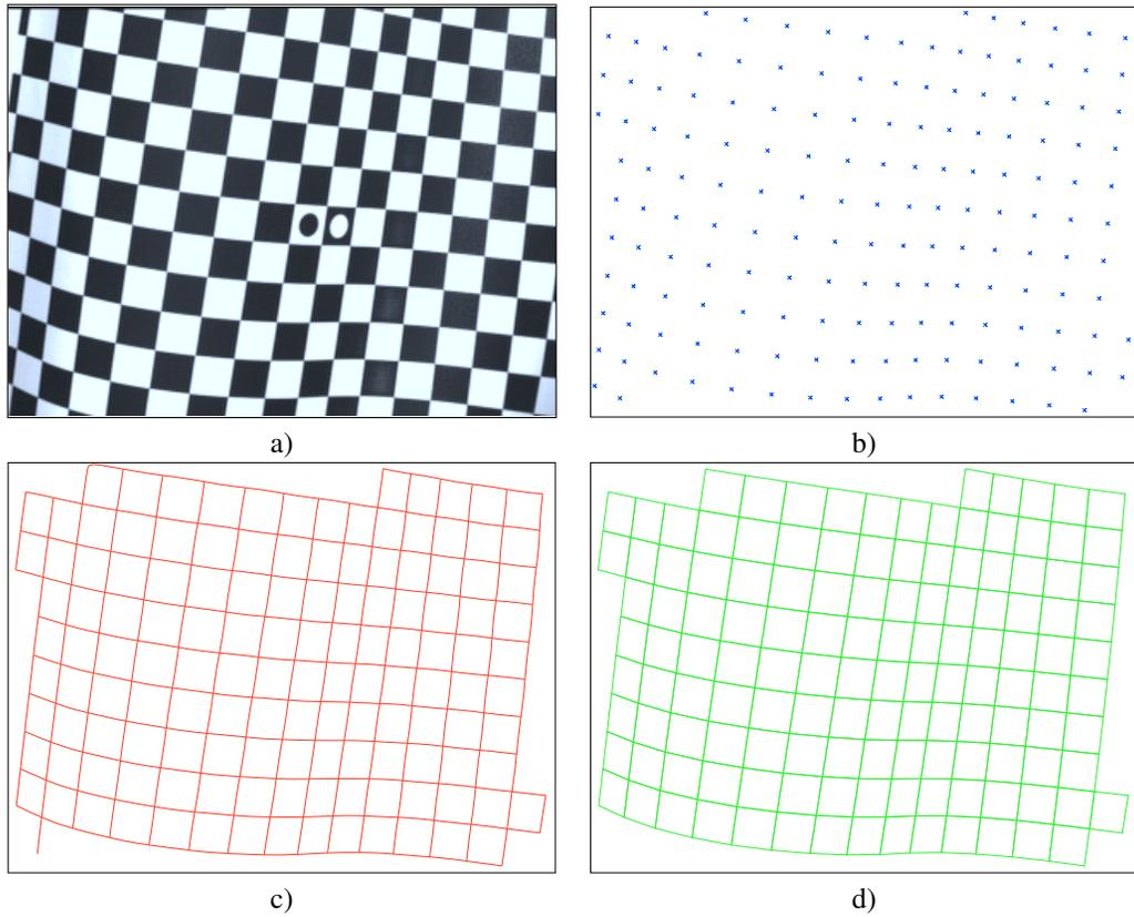
Figure 88: Distorted rectification grid: a) Image; b) extracted corners of the black and white fields; c) lines that connect the corners; d) extracted rectification grid.
