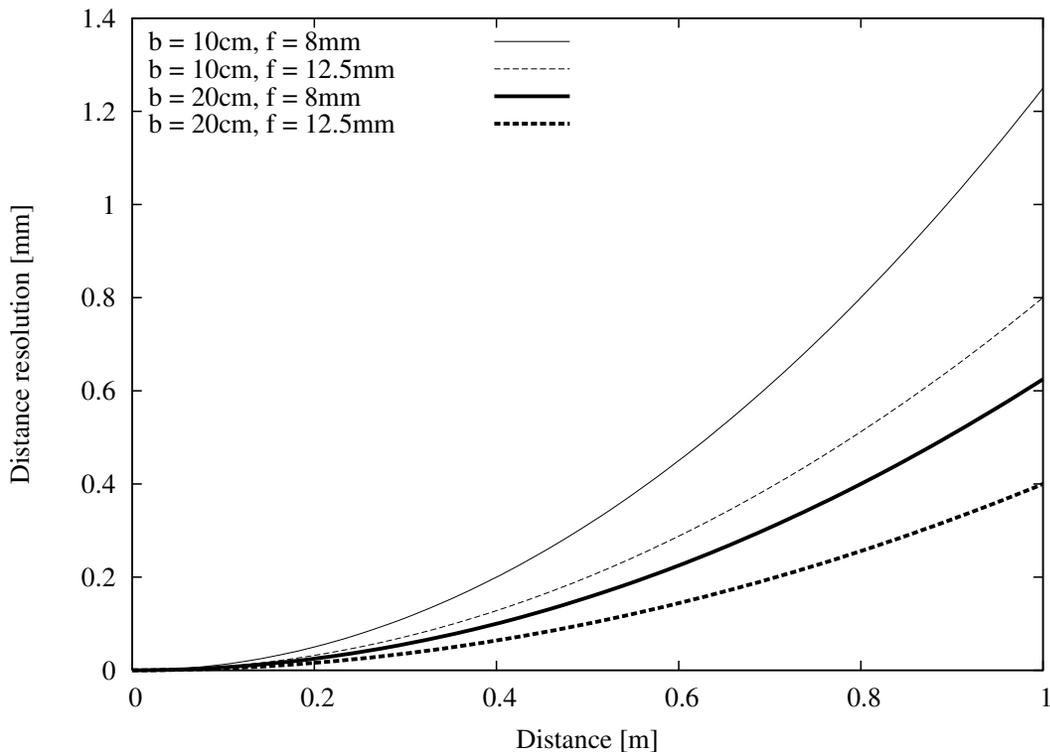
Figure 67: Distance resolution plotted over the distance.
