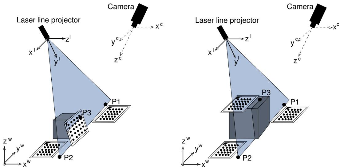
Figure 105: Position of the third point (P3) obtained by (left) tilted calibration plate or (right) translated calibration plate.
