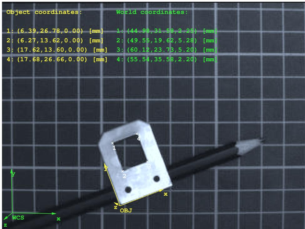
Figure 60: Object coordinates and world coordinates for the four corners of the rectangular hole of the metal part.
