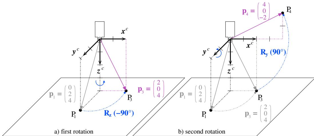
Figure 6: Rotate a point: (a) first around  $z$ -axis; (b) then around  $y$ -axis.
