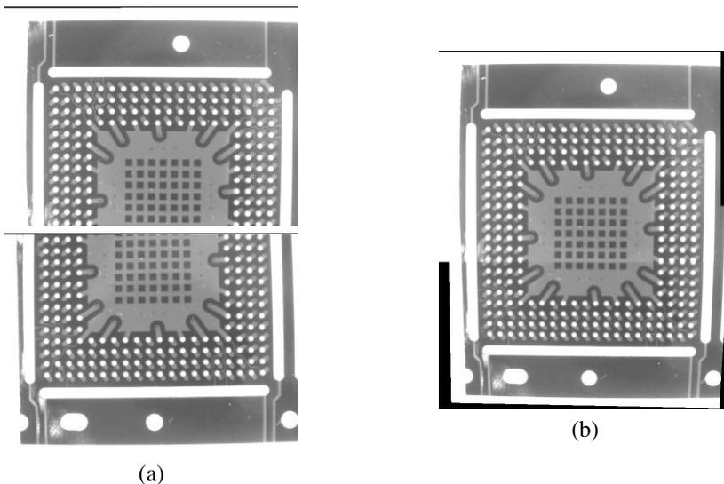
Figure 56: Separate images (a) and mosaic image (b) of a BGA.
