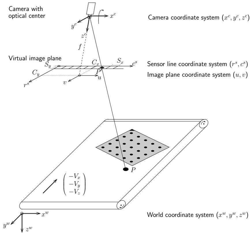
Figure 23: Line scan camera rotated around the x-axis.
