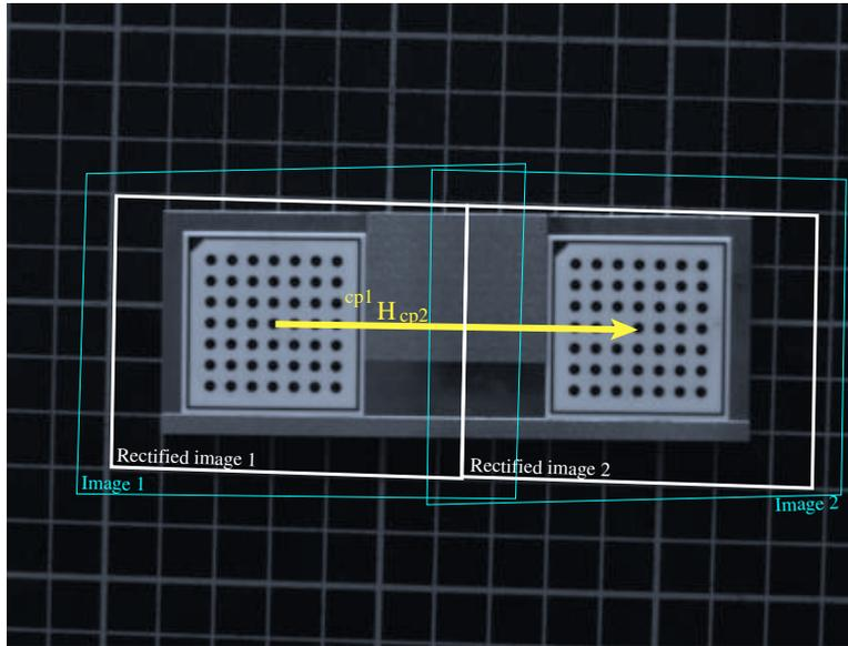
Figure 39: Transformation between the two world coordinate systems, each defined by the respective calibration plate.
