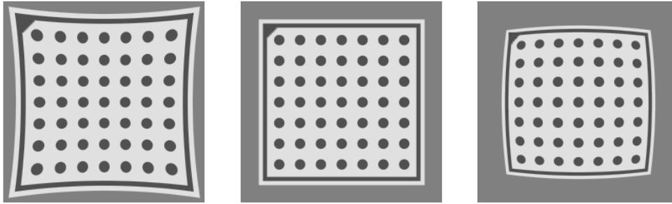
Figure 14: Effect of radial distortions modeled with the division model with  $\kappa > 0$  (left),  $\kappa = 0$  (middle), and  $\kappa < 0$  (right).
