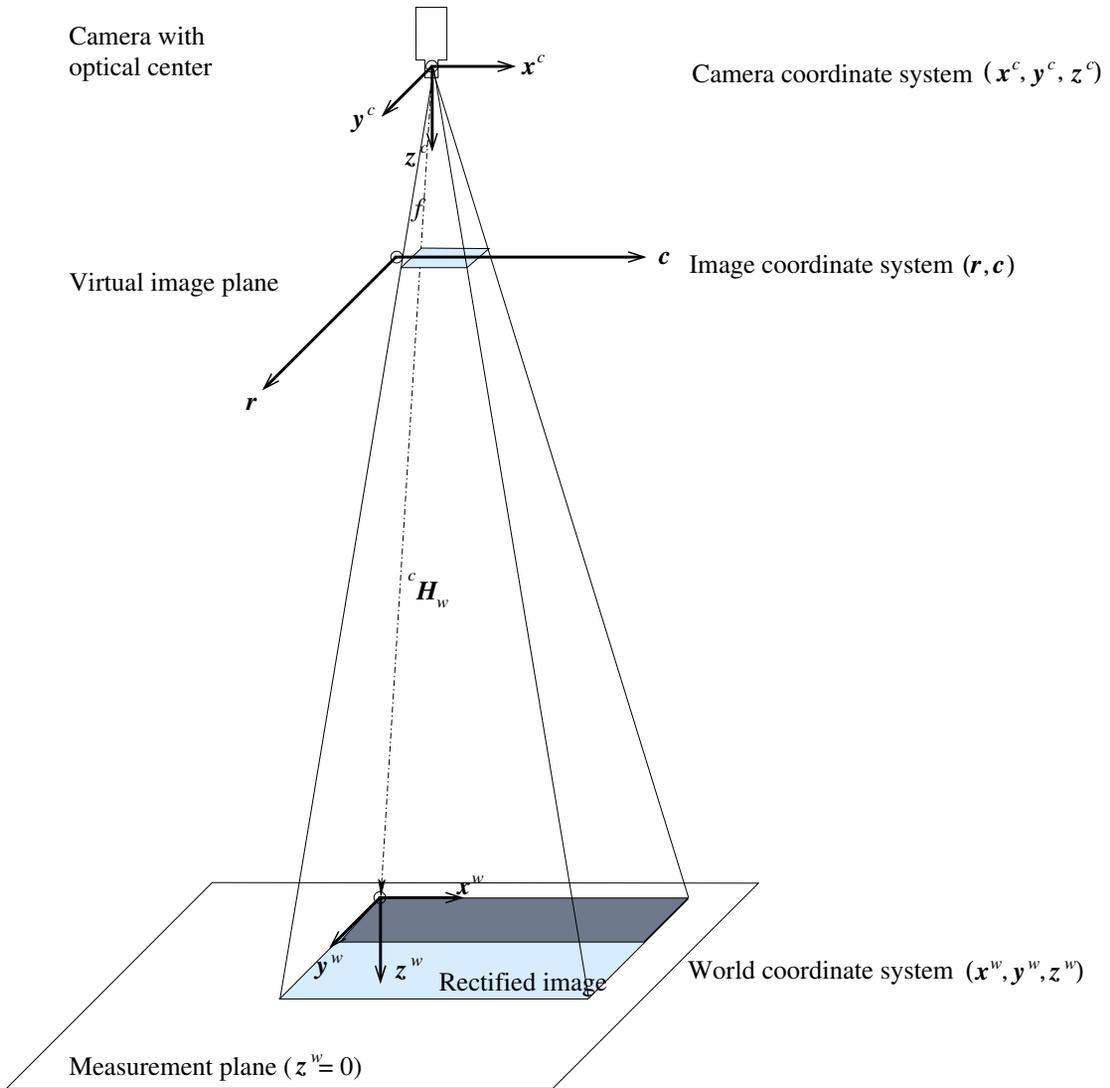
Figure 29: Projection of the image into the measurement plane with part of the rectified image lying outside the image area.
