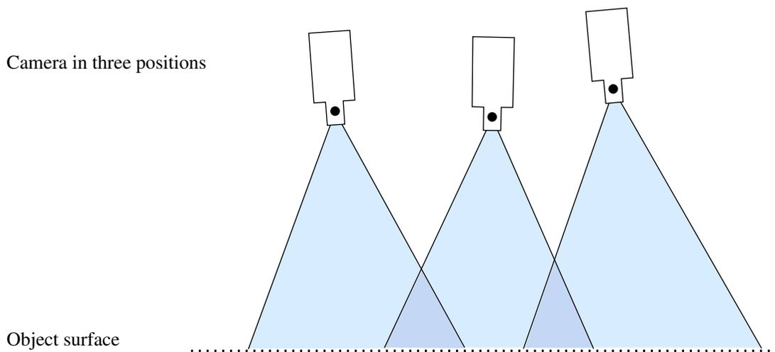
Figure 48: Image acquisition for flat objects.
