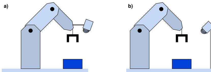
Figure 80: Robot vision scenarios: (a) moving camera, (b) stationary camera.
