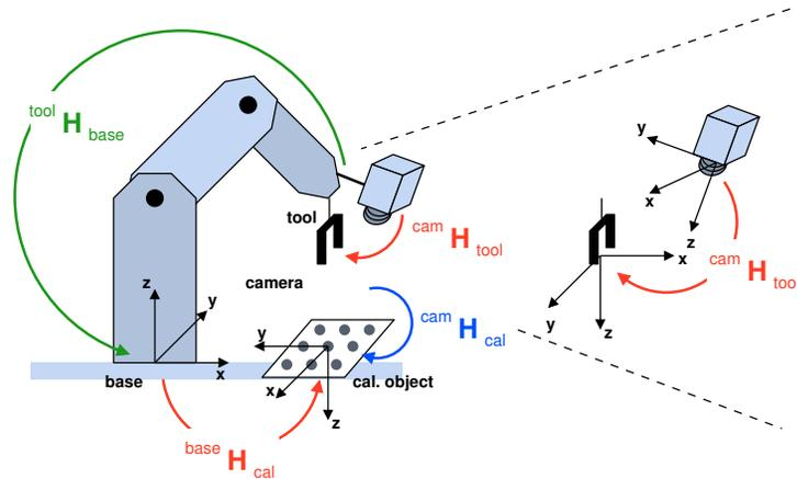
Figure 81: Chain of transformations for a moving camera system.
