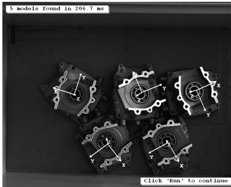
Figure 62: 3D poses of engine parts obtained by a calibrated perspective, deformable matching.
