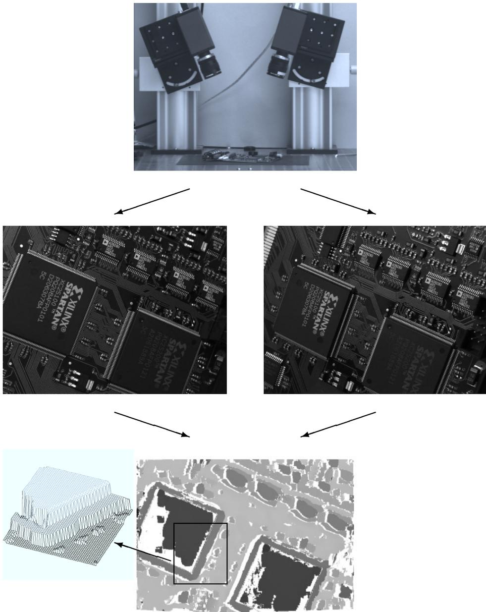
Figure 64: Top: Stereo camera system; Center: Stereo image pair; Bottom: Height map.
