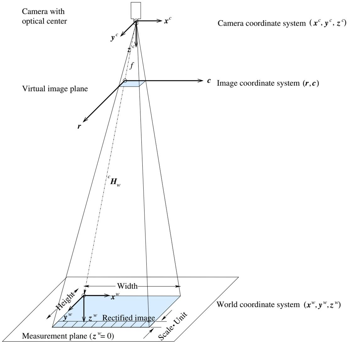
Figure 28: Projection of the image into the measurement plane.
