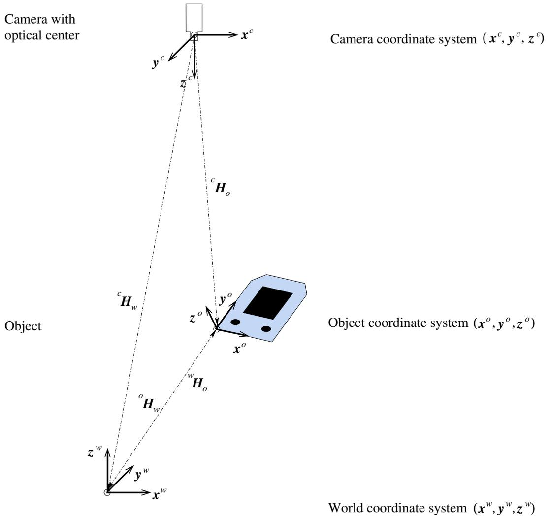
Figure 59: Pose of the object coordinate system and transformation between object coordinates and world coordinates.
