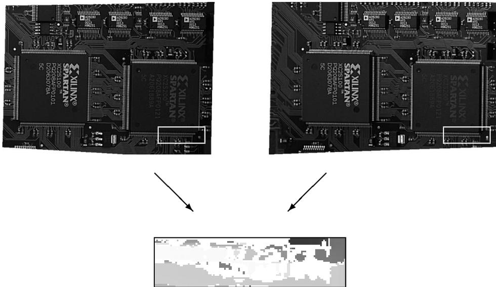
Figure 70: Rectified stereo images with repetitive patterns aligned to the image rows and cutout of the matching result (regions where the matching process failed are displayed white).
