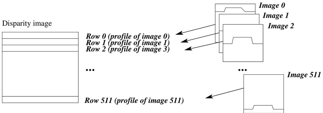
Figure 100: Disparity image: the disparity obtained from each profile (or image, respectively) is stored in a row of the disparity image.
