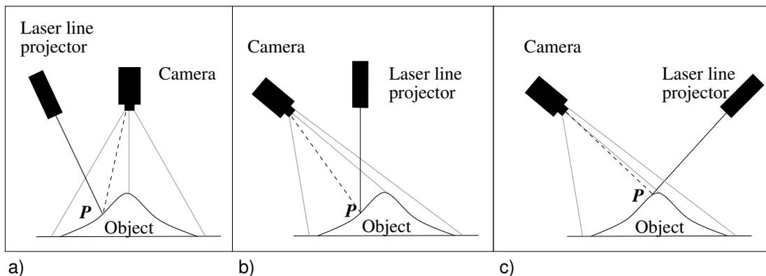
Figure 101: Basic configurations possible for a sheet-of-light measurement setup.
