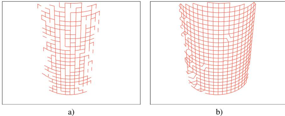
Figure 94: Connecting lines: Parameter `MaxDist` selected a) too small and b) too large.
