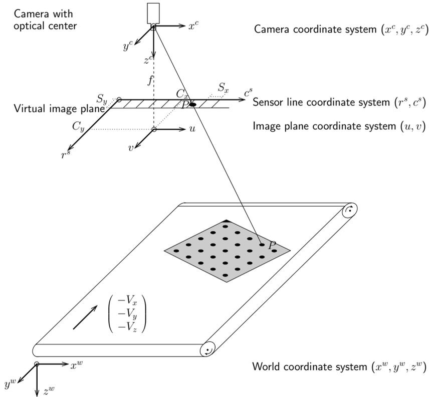
Figure 21: Line scan camera looking perpendicularly onto a conveyor belt.
