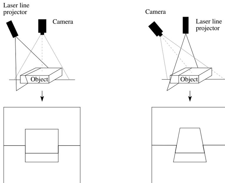
Figure 103: With the camera being orthogonal to the object, an orthogonal projection of the object is possible: (left) orthogonal camera view, (right) perspective view.
