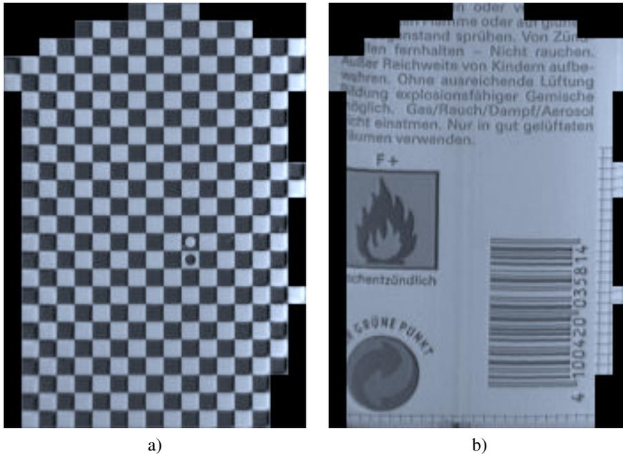
Figure 95: Rectified images: a) Rectification grid; b) object.
