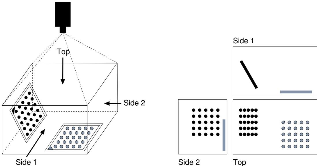
Figure 20: Investigation of the calibration volume: (left) calibration volume with two calibration plate poses and (right) the corresponding distribution of calibration marks when seen from different views. For a good calibration result, the areas without calibration marks (which are especially large in the view from side 1) have to be minimized by a cautious selection of the further calibration plate poses.
