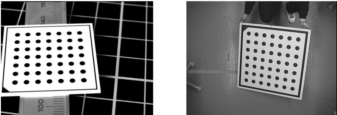
Figure 19: Examples of calibration plates used by HALCON .
