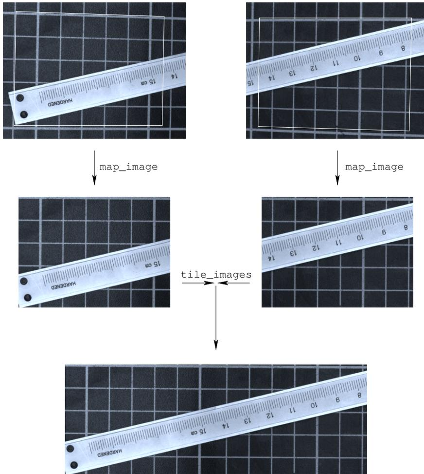
Figure 36: Image rectification and tiling.
