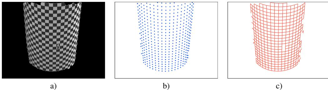
Figure 93: Distorted rectification grid: a) Image reduced to the extracted area of the rectification grid; b) extracted corners of the black and white fields; c) lines that connect the corners.
