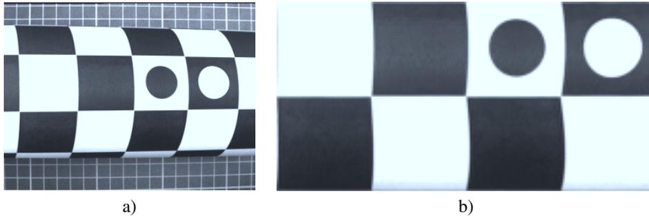
Figure 90: Cylindrical object covered with a very coarse rectification grid: a) Distorted image; b) rectified image.
