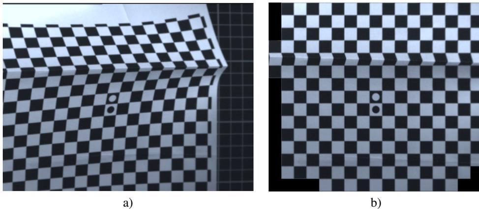
Figure 91: Rectification grid folded across the borders of the black and white fields: a) Distorted image; b) rectified image.
