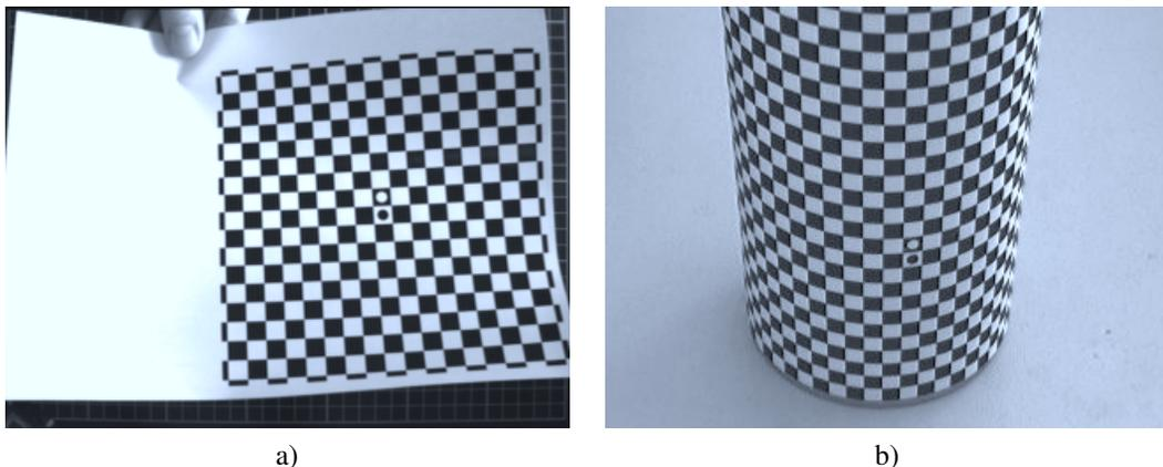
Figure 86: a) Example of a rectification grid. b) Cylindrical object wrapped with the rectification grid.
