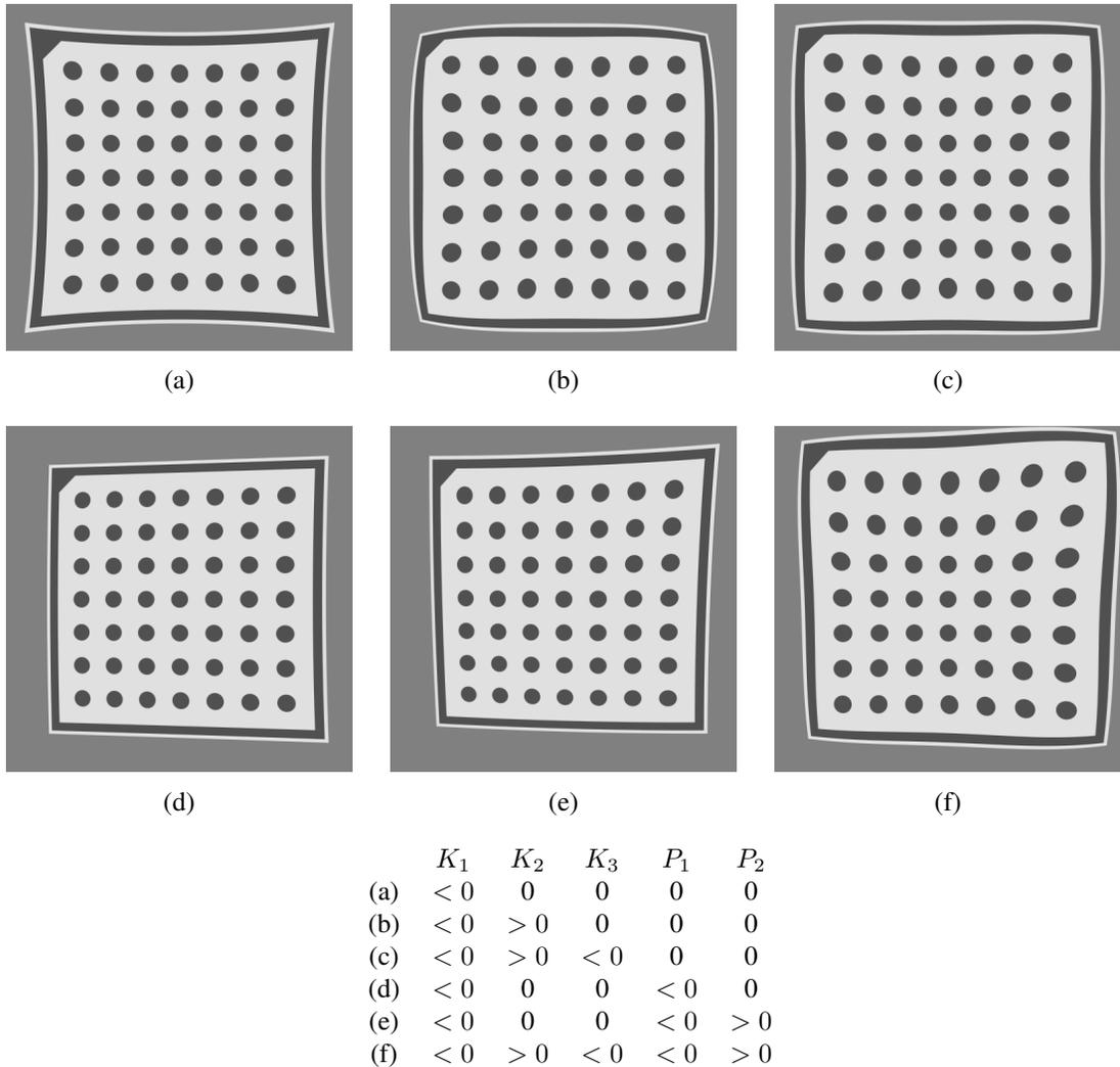
Figure 15: Effect of distortions modeled with the polynomial model with different values for the parameters  $K_1$ ,  $K_2$ ,  $K_3$ ,  $P_1$ , and  $P_2$ .
