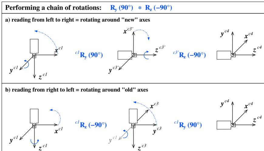
Figure 8: Performing a chain of rotations (a) from left to the right, or (b) from right to left.
