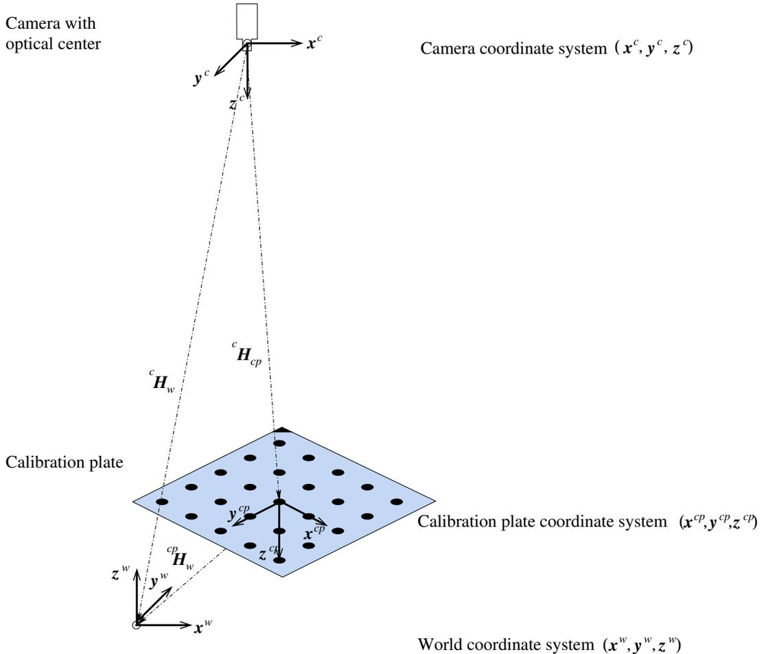
Figure 58: Determination of the pose of the world coordinate system.
