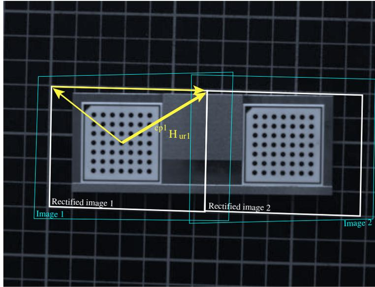
Figure 38: Definition of the upper right corner of the first rectified image.
