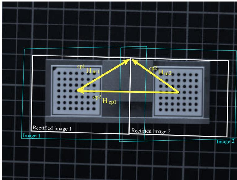
Figure 40: Definition of the upper left corner of the second rectified image.
