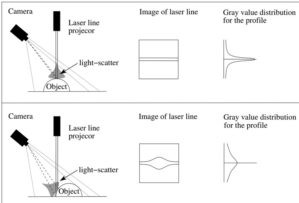
Figure 111: Curved surfaces with a small radius of curvature and surfaces with a significant slope lead to a broadening of the light line and thus to a low score: (top) small influence of curvature, (bottom) large influence of curvature.
