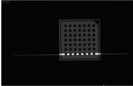
Figure 106: The white parts of a HALCON calibration plate show a very broad laser line because of volume scattering.
