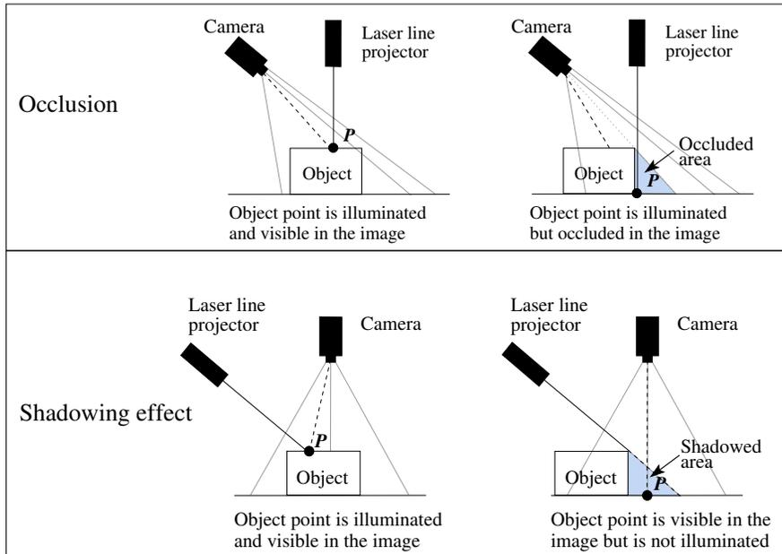
Figure 104: Problems that have to be considered before selecting the measurement setup: (top) occlusions and (bottom) shadowing effects.
