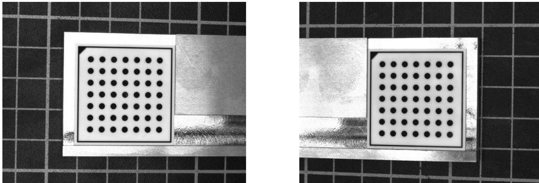
Figure 35: Calibration images for two-camera setup.
