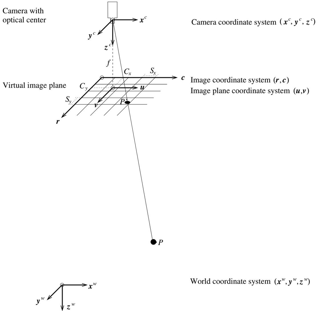
Figure 12: Image plane and virtual image plane.
