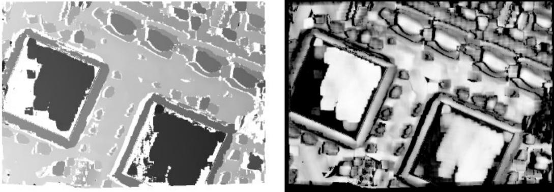
Figure 76: Disparity image (left) and score image (right).
