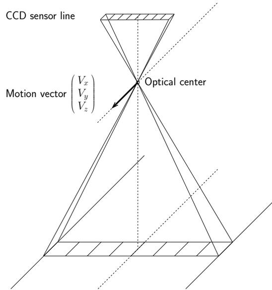
Figure 16: Principle of line scan image acquisition.
