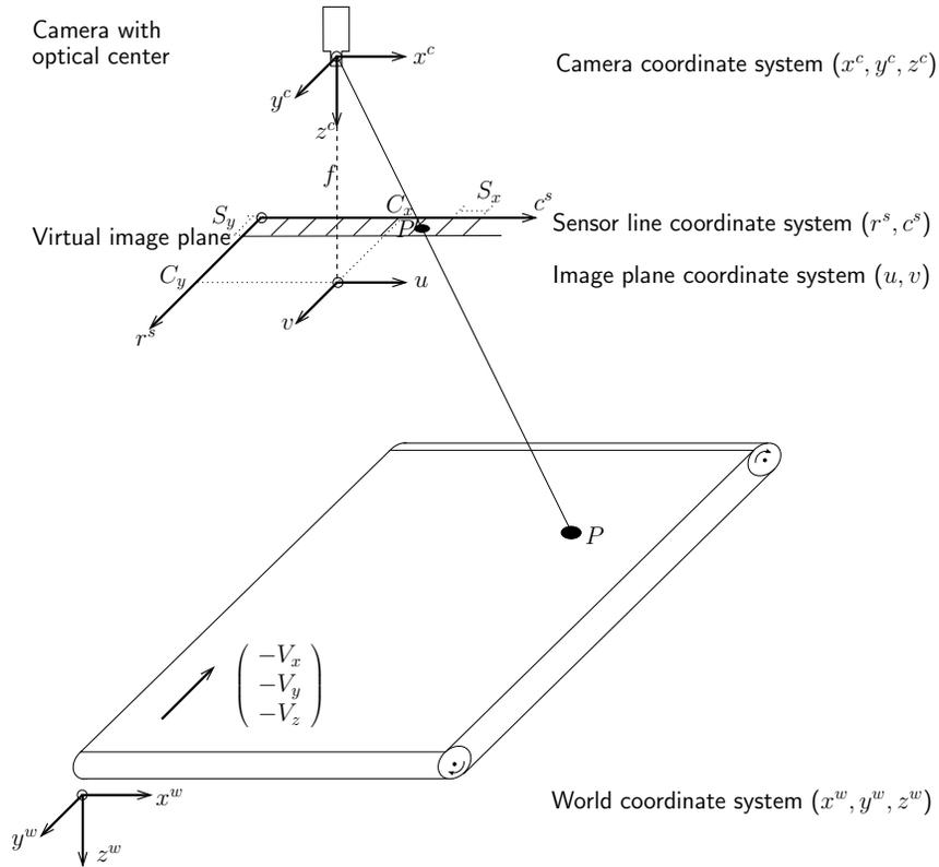
Figure 17: Coordinate systems in regard to a line scan camera.
