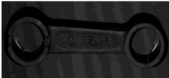
Figure 112: Result of uncalibrated sheet-of-light measurement: score image (score\_type set to 'width', i.e., bright parts indicate artifacts).
