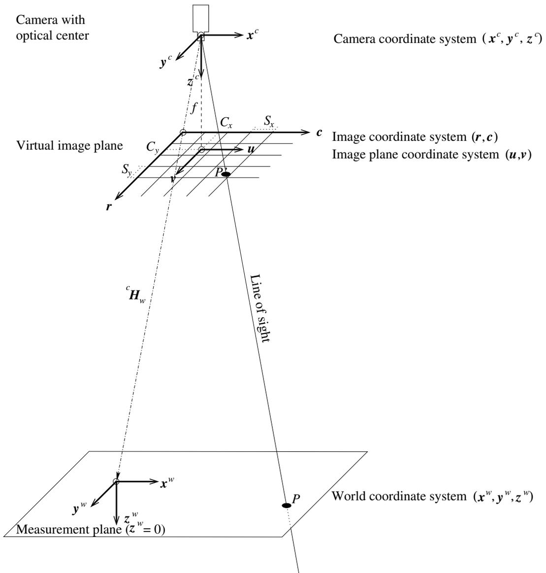
Figure 26: Intersecting the line of sight with the measurement plane..
