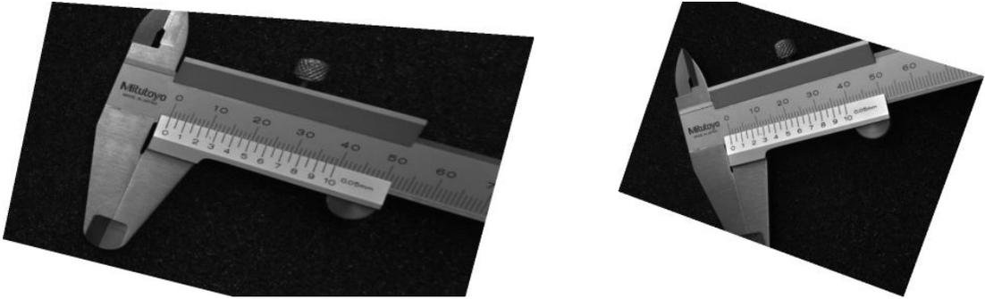
Figure 74: Incorrectly rectified stereo images.
