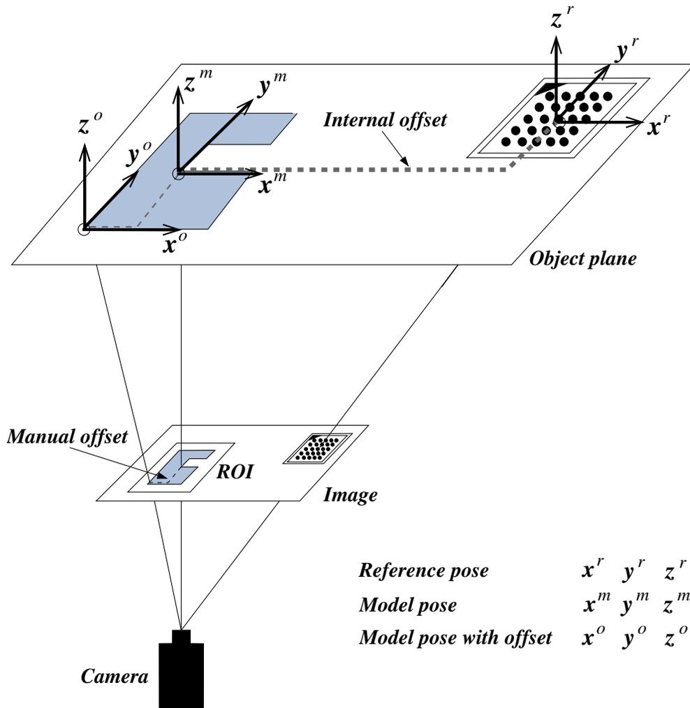
Figure 61: Internal and manual offset: the offset from the reference pose to the model pose is calculated automatically from the reference pose, the internal camera parameters, and the template image. An additional offset can be applied manually and is defined in image coordinates.
