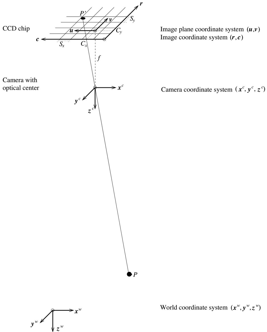
Figure 11: Perspective projection by a pinhole camera.
