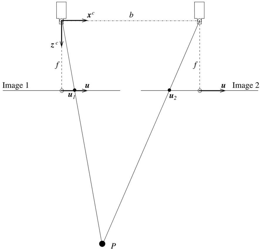
Figure 65: Vertical section of a binocular stereo camera system.
