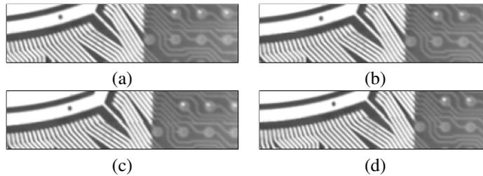
Figure 57: Seam between image 5 and image 10 for different classes of transformations: (a) projective, (b) affine, (c) similarity, and (d) rigid.
