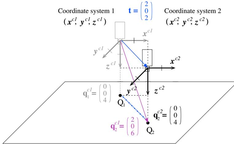
Figure 5: Translating a coordinate system (and point).
