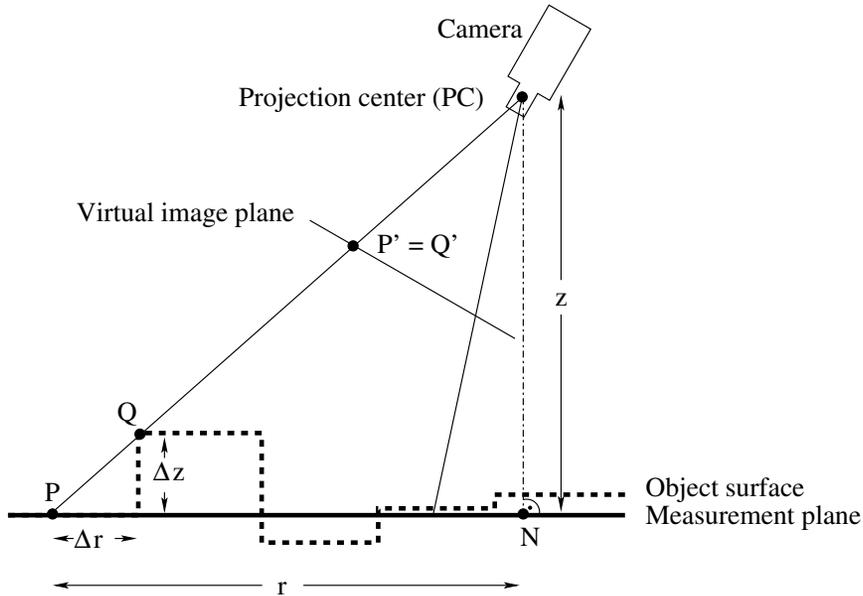
Figure 31: Displacement  $\Delta r$  caused by a deviation of the object surface from the measurement plane.
