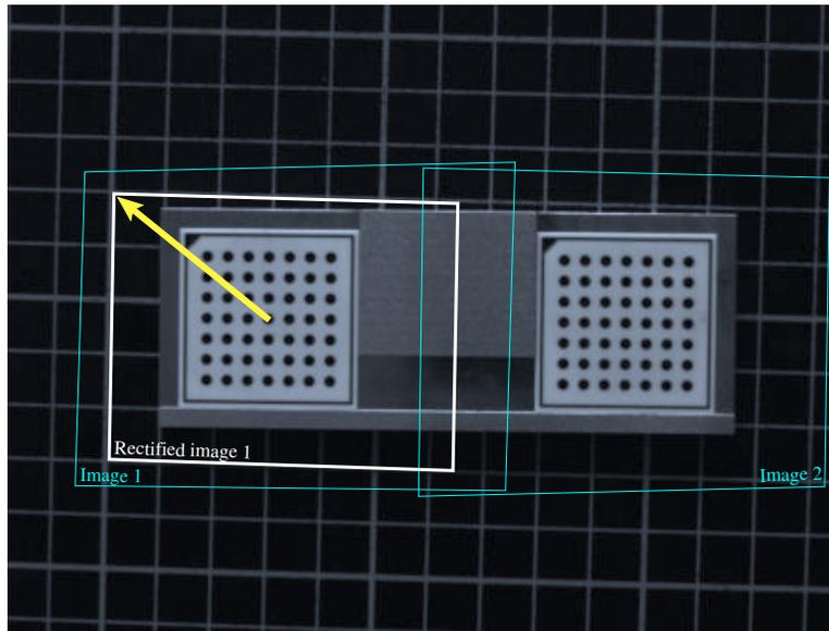
Figure 37: Definition of the upper left corner of the first rectified image.
