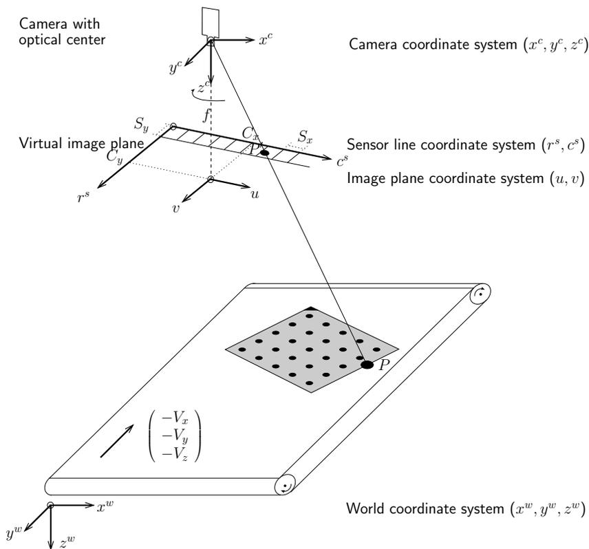
Figure 22: Line scan camera rotated around the optical axis.
