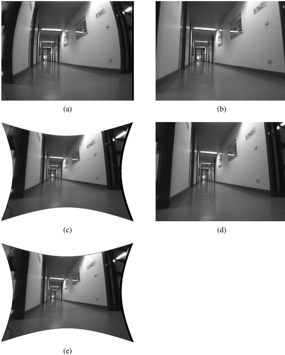
Figure 30: Eliminating radial distortions: (a) The original image; (b) the image rectified by setting  $\kappa$  to zero; (c) the image rectified with mode *'fullsize'*; (d) the image rectified with mode *'adaptive'*; (e) the image rectified with mode *'preserved\_resolution'*.
