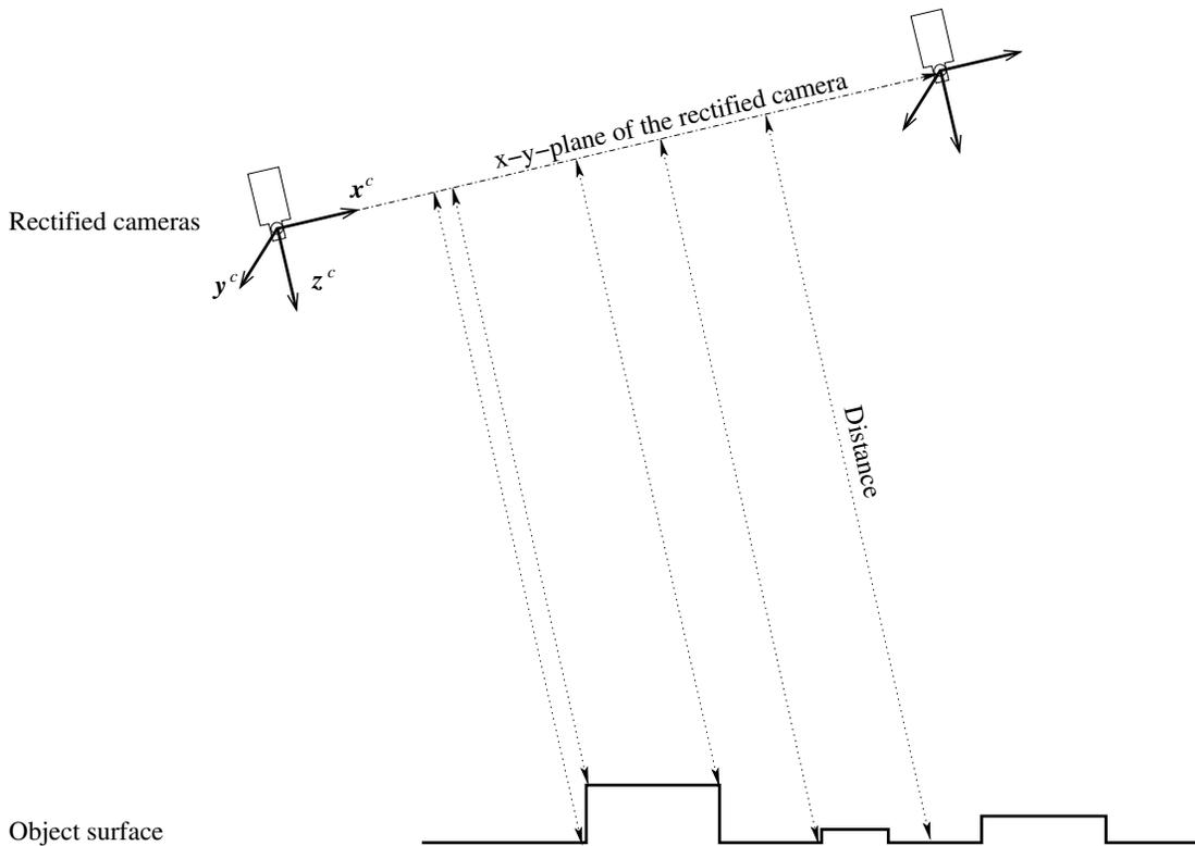
Figure 78: Distances of the object surface from the  $x$ - $y$ -plane of the coordinate system of the first rectified camera.
