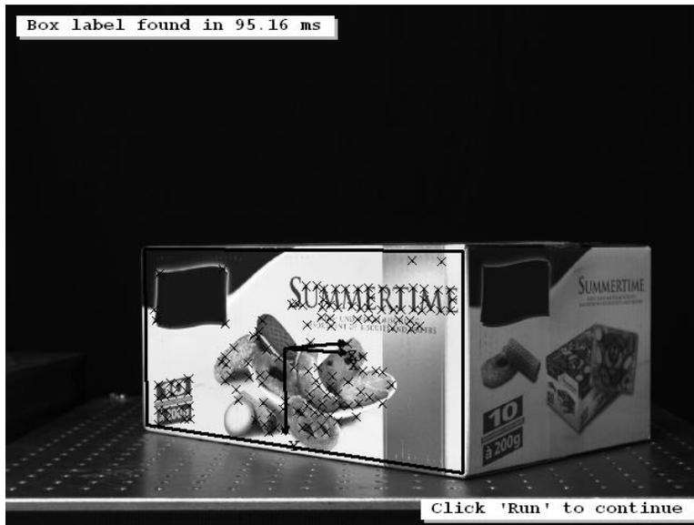
Figure 63: 3D pose of a cookie box label obtained by a calibrated descriptor-based matching.
