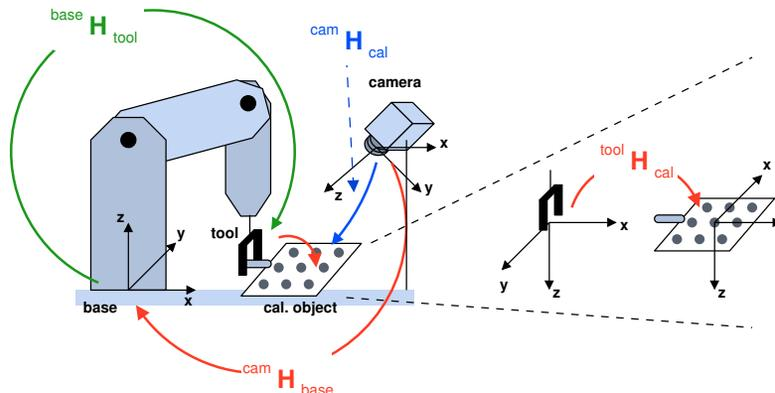
Figure 82: Chain of transformations for a stationary camera system.
