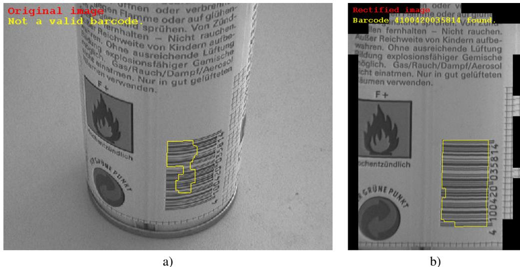
Figure 85: Cylindrical object: a) Original image; b) rectified image.
