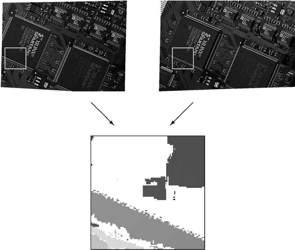
Figure 69: Rectified stereo images and matching result of the correlation-based stereo in a poorly textured area (regions where the matching process failed are displayed white).
