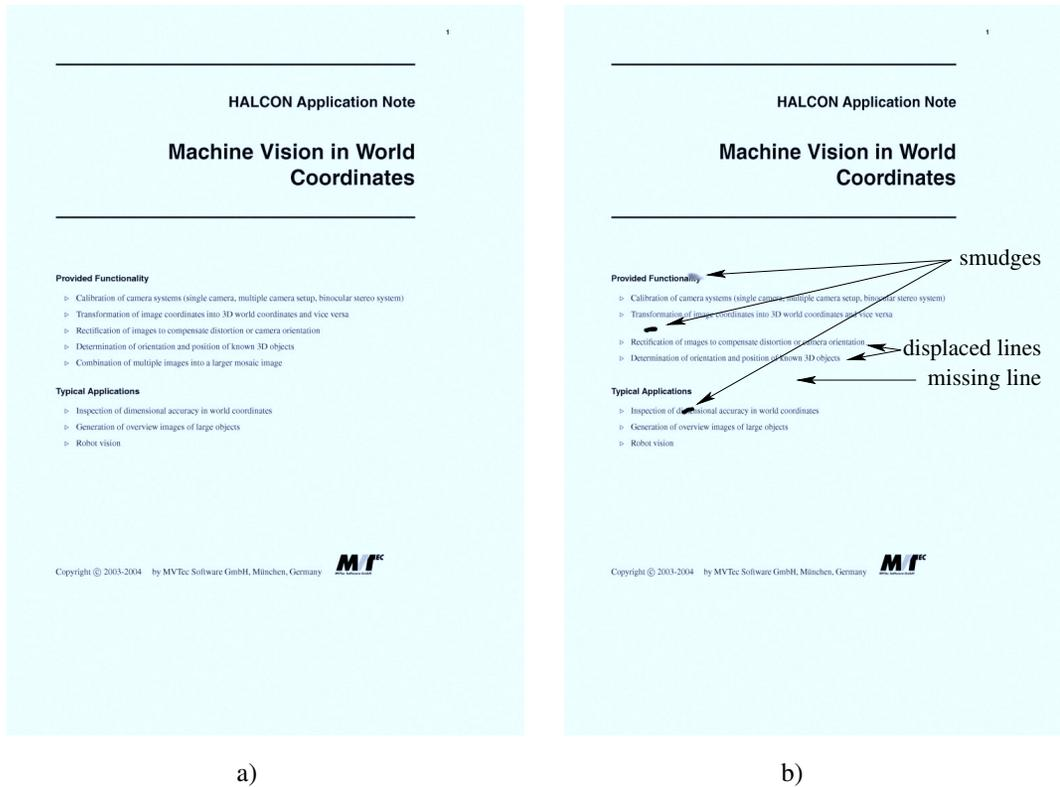
Figure 96: Images of one page of a document: a) Reference image; b) test image that must be checked.
