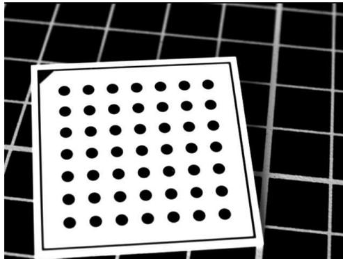
Figure 18: The HALCON calibration plate.
