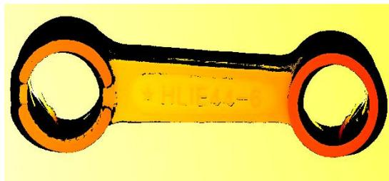
Figure 110: Result of uncalibrated sheet-of-light measurement: disparity image.
