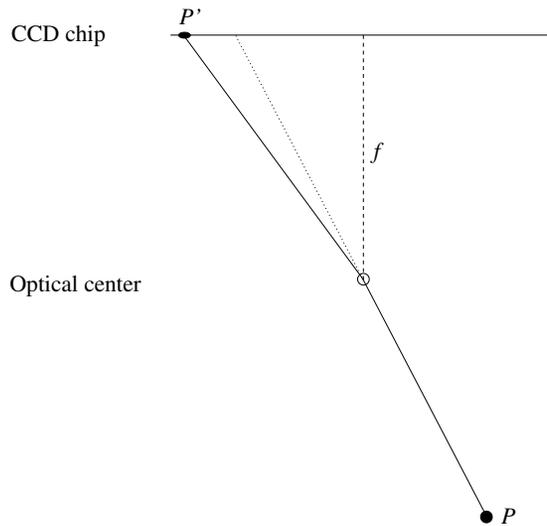
Figure 13: Schematic illustration of the effect of the lens distortion.
