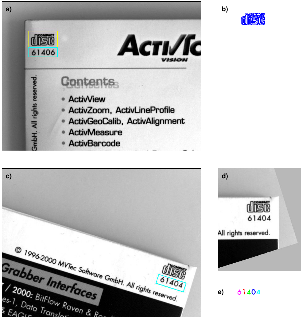
Figure 21: Rectifying the search results: a) ROIs for the model and for the number extraction; b) the model; c) number ROI at matched position; d) rectified search image (only relevant part shown); e) extracted numbers.
