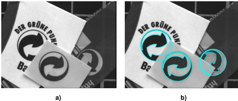
Figure 9.5: Using template matching to locate rotated and scaled objects: (a) search image; (b) matches.
