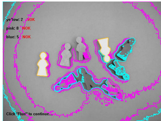
Figure 13.8: Poor classification result when only using the gray scale image.
