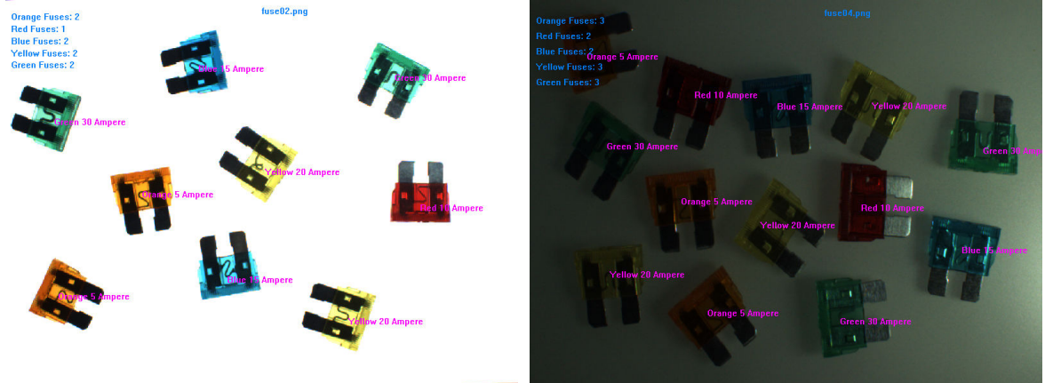
Figure 13.6: Simple classification of fuses by color with varying illumination.
