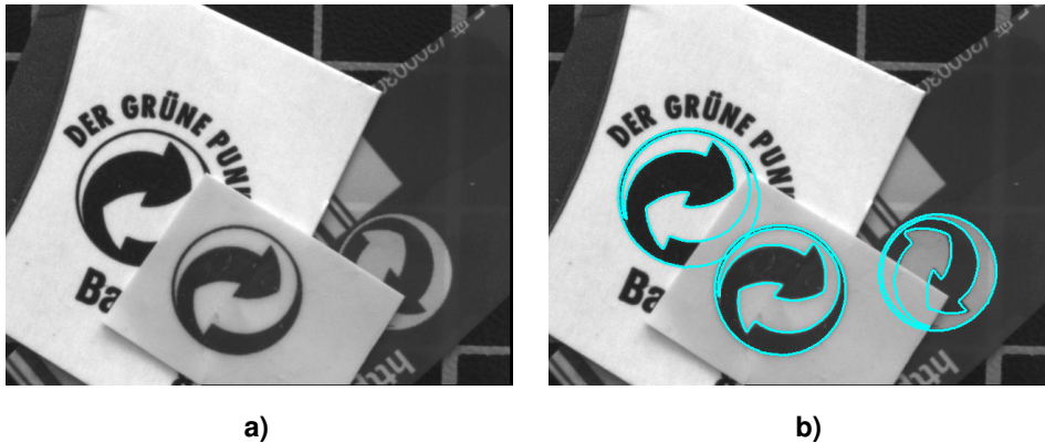
Figure 3.21: Using template matching to locate rotated and scaled objects: (a) search image; (b) matches.
