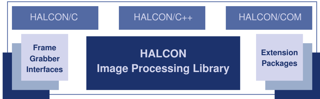
Figure 2.2: Basic architecture of HALCON.
