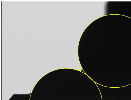
Figure 4.8: Fitting circles to the contours of the tool.
