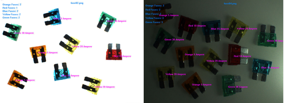
Figure 3.27: Simple classification of fuses by color with varying illumination.
