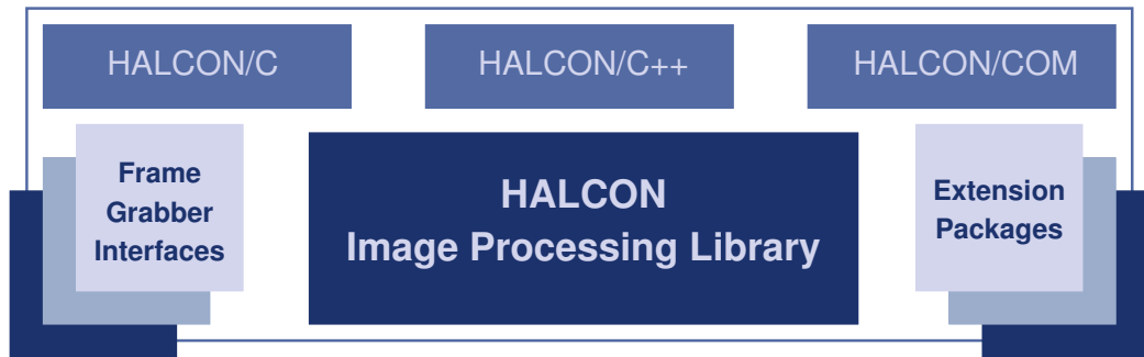
Figure 2.2: Basic architecture of HALCON.
