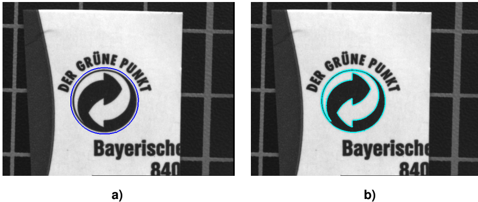
Figure 3.20: Creating a model for template matching: (a) ROI for the template region; (b) model contours.
