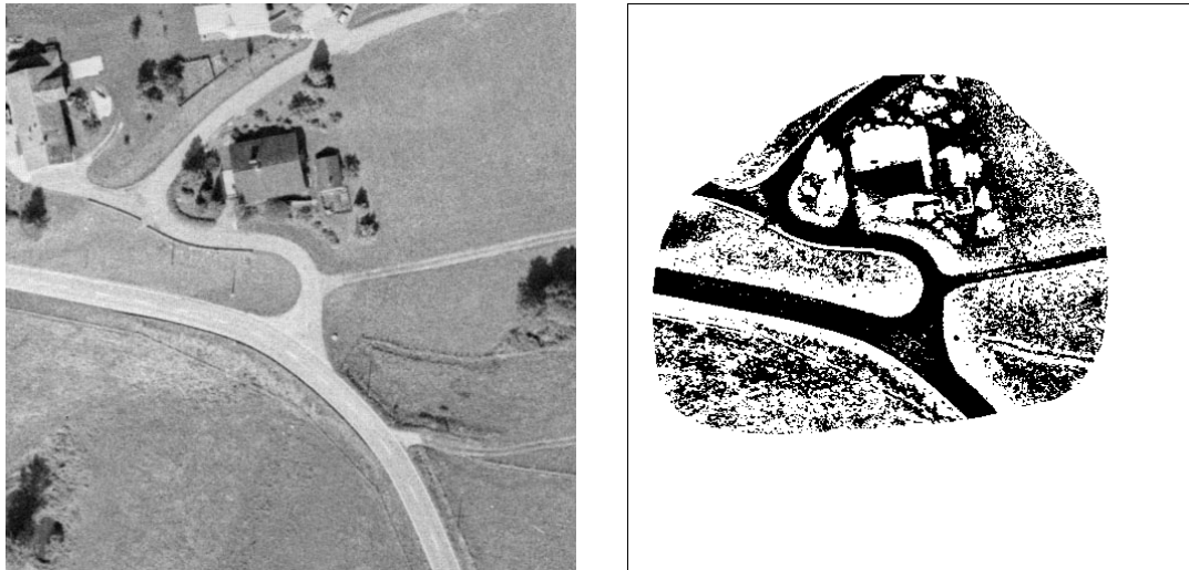
Figure 2.6: On the left side the input image ( mreut.tiff ), and on the right side the segmented regions in the selected image domain.
