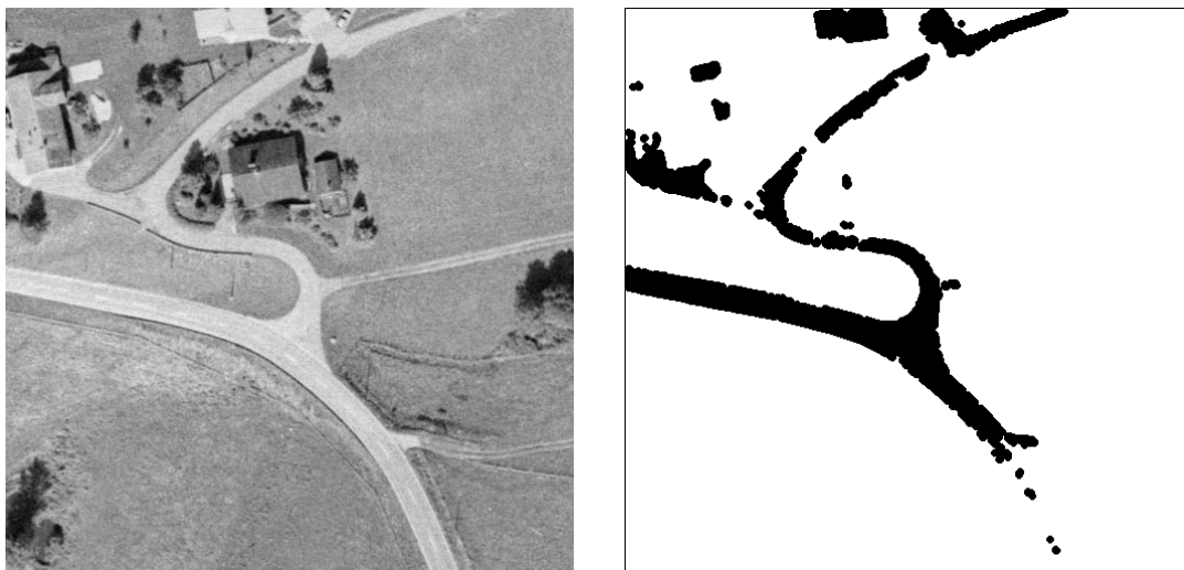
Figure 2.2: On the left the input image ( mreut.tiff ), and on the right the region after the opening ( open ).
