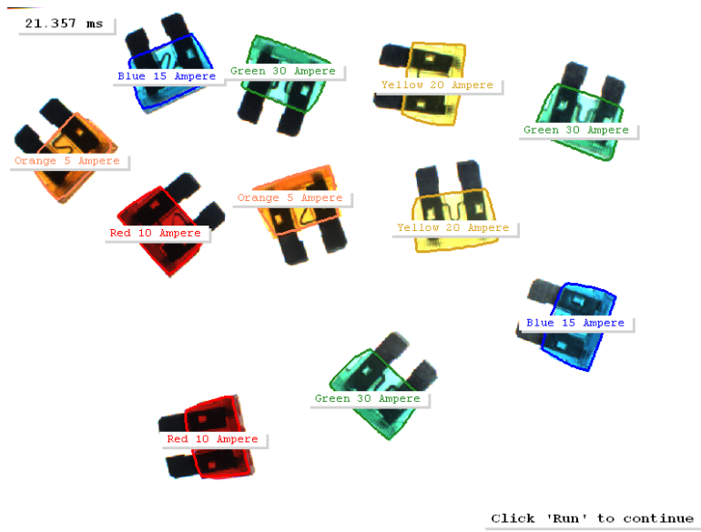
Figure 6.6: Fuses of different color are segmented using a LUT-accelerated GMM classifier.
