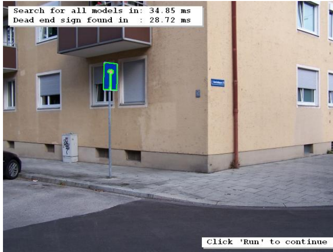
Figure 9.12: A dead end road sign is located via uncalibrated perspective deformable matching.
