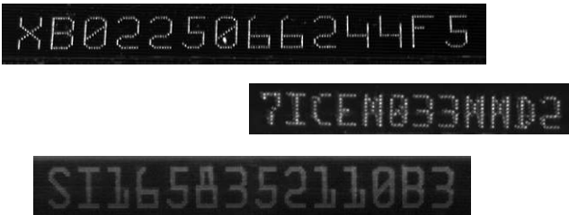
Figure 17.20: Examples for SEMI font. Note that these images were inverted before the training was applied! That is, this font is nevertheless pretrained only for dark on light symbols.
