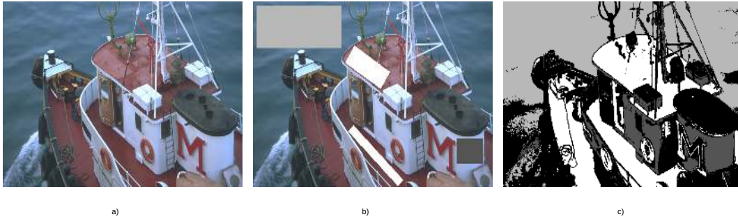
Figure 12.1: Segmentation of a color image: (a) original image, (b) sample regions for the classes Sea (light gray), Deck (white), and Walls (gray), (c) regions returned by the classification (black marks the rejected regions).
