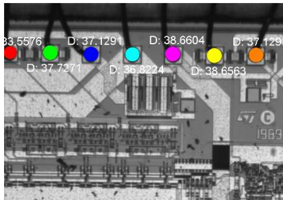
Figure 4.7: Measuring the diameter of ball bonds.
