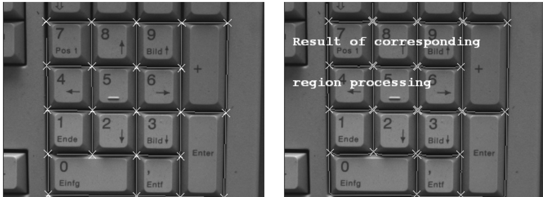
Figure 5.14: Get junction points: (left) lines fitted into linear contours and the junction points of the grid separating the keys, (right), skeleton and irregular junction points obtained by region processing.
