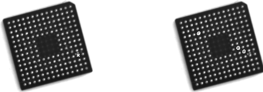
Figure 5.24: Irregularities of a BGA: (left) missing ball marked by a cross, (right) balls with center positions that deviate from the reference positions marked by ellipses.
