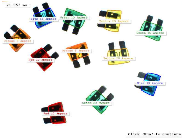
Figure 6.6: Fuses of different color are segmented using a LUT-accelerated GMM classifier.
