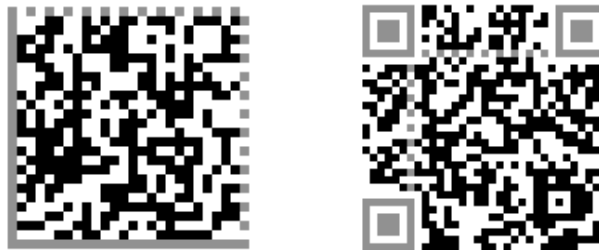
Figure 1.2: Types of matrix codes (finder patterns are marked in gray): (left) Data Matrix ECC 200 and (right) QR Code.
