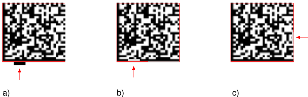
Figure 6.4: Quality grades with value 0 for fixed pattern damage: (a) damaged quiet zone, (b) damage at the L-shape of the finder pattern, and (c) damage at the alternating side of the finder pattern.
