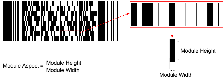
Figure 3.9: Module aspect ratio for PDF417.
