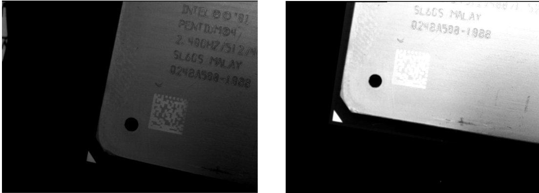
Figure 3.2: Images with different contrast values for training the 2D data code model.
