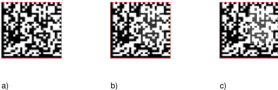
Figure 6.2: Quality grades for the modulation: (a) 4, (b) 2, and (c) 0.
