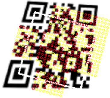
Figure 5.11: The symbol candidate is related to two position detection patterns and does not fit the actual symbol outline.
