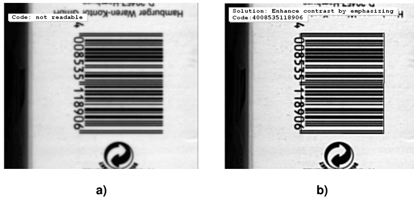
Figure 15.5: a) A blurry bar code cannot be decoded. b) After enhancing the contrast, the code can be read.
