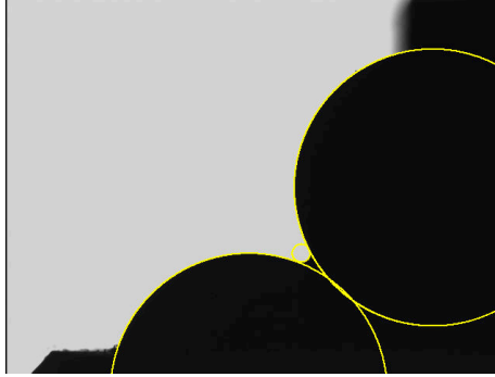
Figure 3.4: Fitting circles to the contours of the tool.
