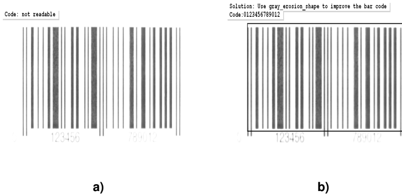
Figure 15.9: a) An overexposed bar code b) gray_erosion_shape reverses the effect of the overexposure.
