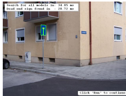
Figure 9.12: A dead end road sign is located via uncalibrated perspective deformable matching.
