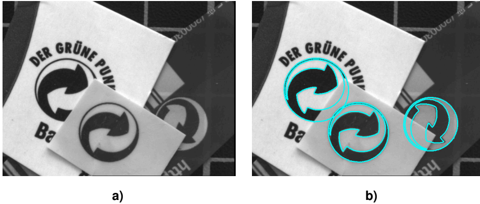
Figure 9.5: Using matching to locate rotated and scaled objects: (a) search image; (b) matches.
