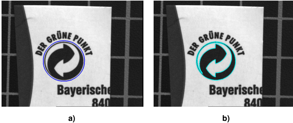
Figure 9.4: Creating a model for matching: (a) ROI for the template region; (b) model contours.
