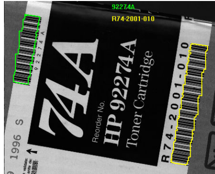
Figure 3.16: Detected bar codes.
