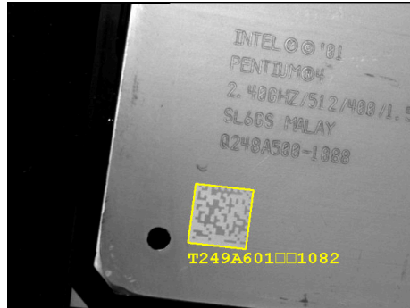
Figure 4.2: Decoded data code.
